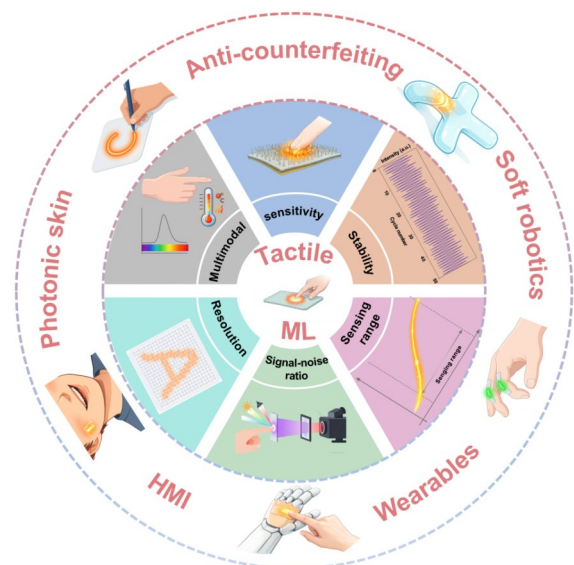
图1 力致发光触觉传感的关键性能指标与应用。 Fig.1 Key metrics and representative applications of mechanoluminescent materials for tactile sensing.
